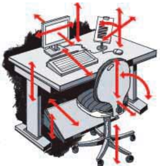
Ill. 3: The individual elements of a computer workstation must be adjustable and correctly positioned.
