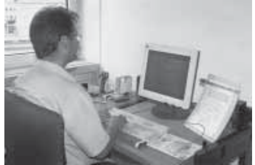
Ill. 1: Correct positioning of the screen (at right angles to the source of light).
